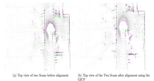
FIGURE 3.2: Left: Two point clouds before alignment, Right: Point Clouds after alignment using the ICP algorithm
