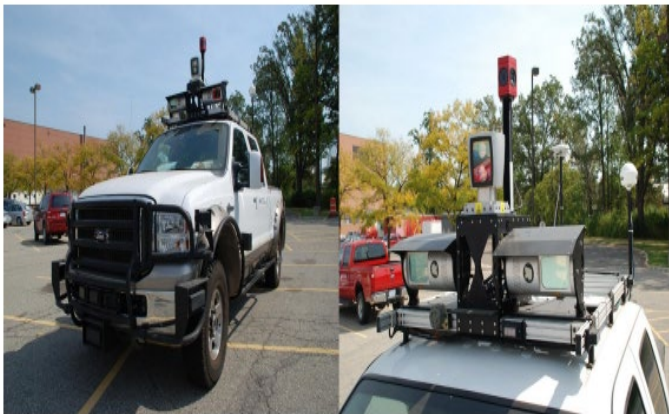
FIGURE 1.1: Test Vehicle (Left). 3D lidar and omni-directional camera system mounted on the test vehicle (Right) [24].
